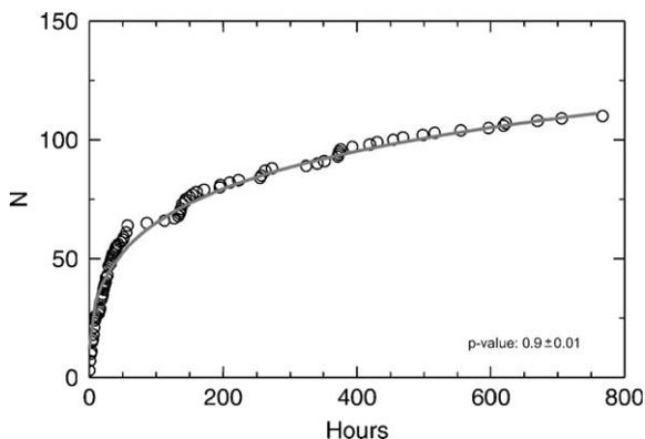
Fig. 7. p-value for the aftershock sequence of the 8 October 2005 Muzaffarabad earthquake using 110 aftershocks in magnitude range of 5 to 6.3.
