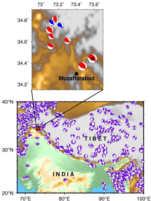
Fig. 4. Focal mechanism solutions of earthquakes in the Himalaya, Tibet, Pamir and Hindukush regions, from the Harvard CMT catalogue. Inset: a close up of the Muzaffarabad region indicating the focal mechanisms of the 8 October 2005 Himalayan earthquake and its aftershocks. The blue coloured mechanisms correspond to earthquakes prior to the 8 October 2005 event.
