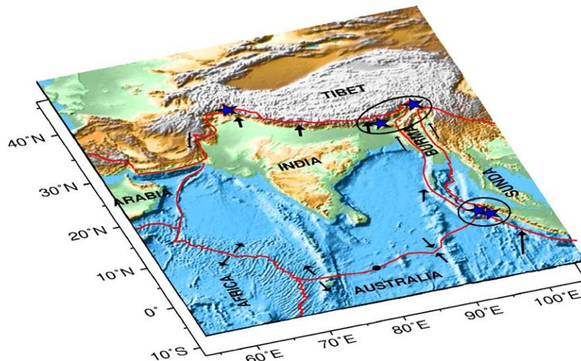
Fig. 9. A cartoon depicting the tectonic scenario of the Indian plate and the neighbouring plates. The vectors represent plate motion velocities along the Indian plate margins, computed using NUVEL-1A model (DeMets et al., 1994). Black circle represents the Euler pole of rotation of the India–Australia plate pair. Presence of great earthquakes close to the quadruple plate junctions is noteworthy.
