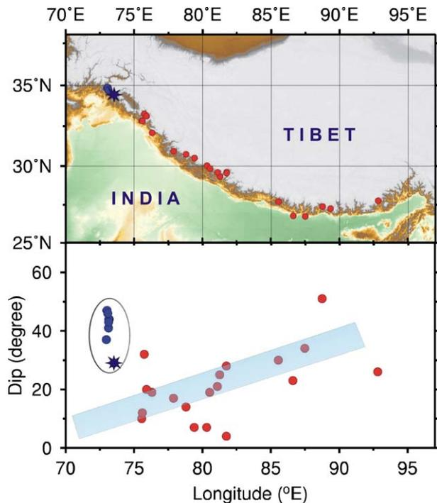
Fig. 5. Variation of the dip angles of the shallow northward dipping fault planes of Himalayan earthquakes, from west to east. Note that the recent Muzaffarabad earthquake of 8 October 2005 and its aftershocks, all have steeply dipping fault planes and fall in a cluster separate from the observed average trend for typical Himalayan earthquakes.
